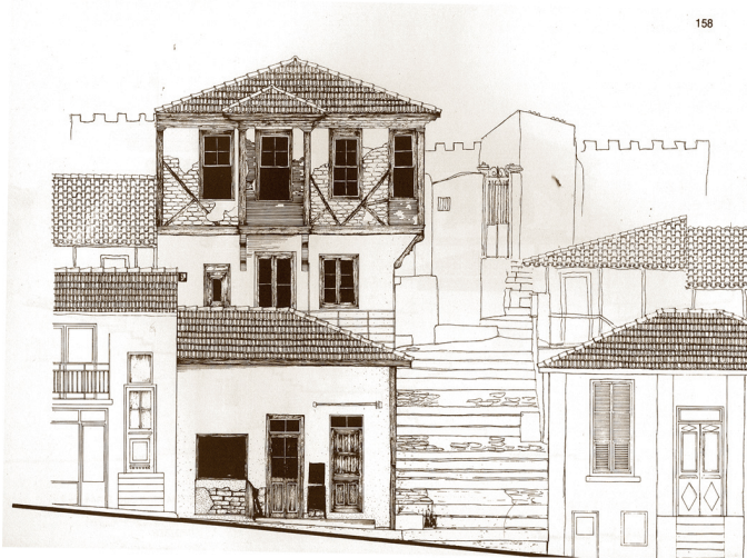
A view, from Acropolis St. of the side of 1-3 Sylla St. The survey shows the timber diagonals which prop the overall frame, along with the mud block infill.
